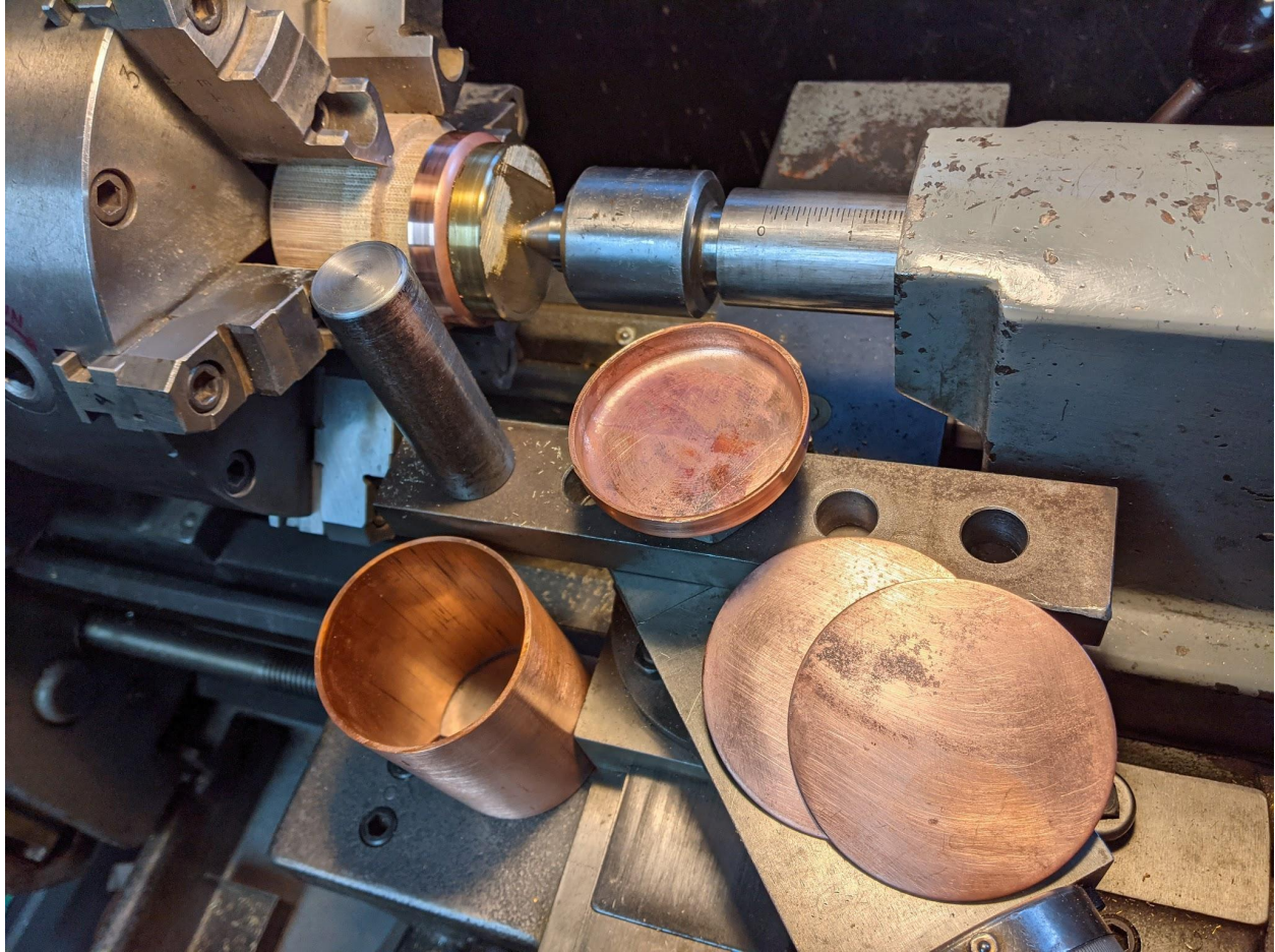
The brass piece is the pressure plate. New blanks and a finished part are shown.
