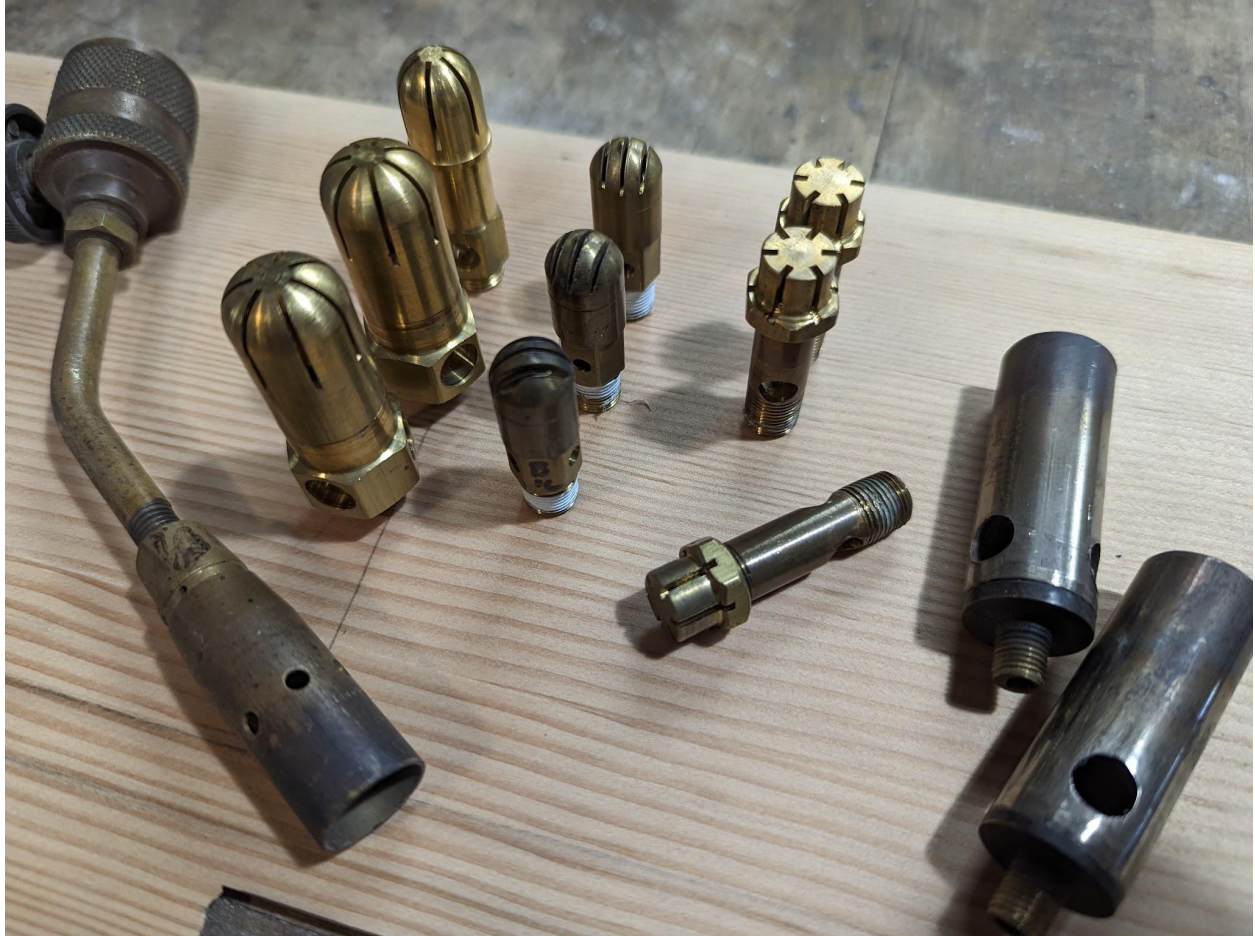
A group of burner jets, star and fan pattern. With a couple jet burners and a propane torch head as well.
